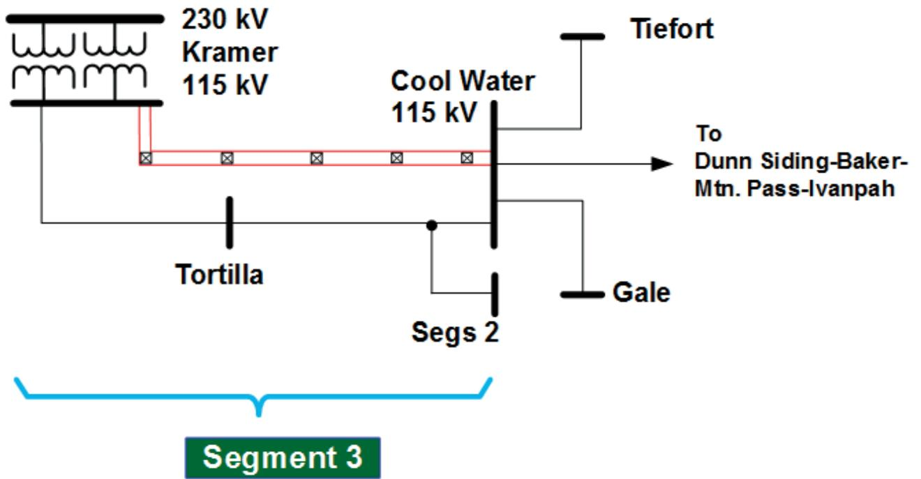
SYSTEM TOPOLOGY--DERATE EXISTING CIRCUIT IN SEGMENT 3S, REMEDIATE REMAINING GO 95 DISCREPANCIES IN SEGMENT 3S, AND REBUILD SEGMENT 3N WITH DOUBLE-CIRCUIT POLE LINE
