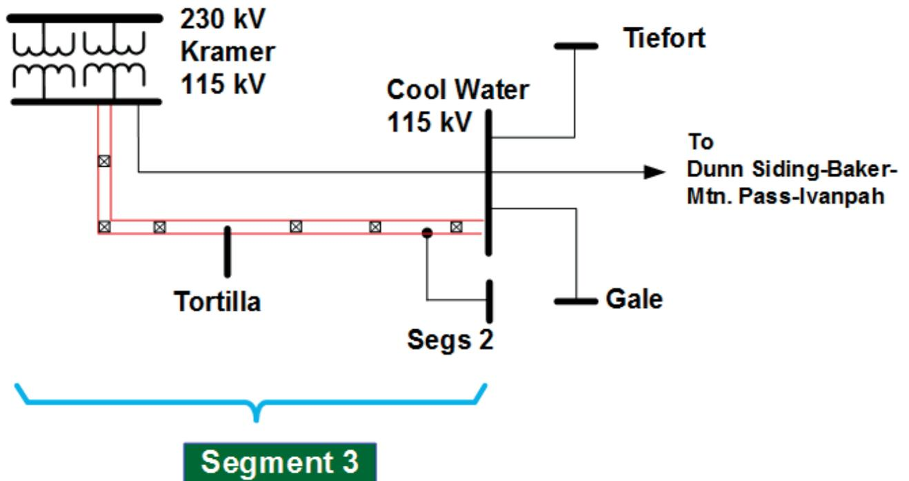
SYSTEM TOPOLOGY--DERATE EXISTING CIRCUIT IN SEGMENT 3N, REMEDIATE REMAINING GO 95 DISCREPANCIES IN SEGMENT 3N, AND REBUILD SEGMENT 3S WITH DOUBLE-CIRCUIT POLE LINE
